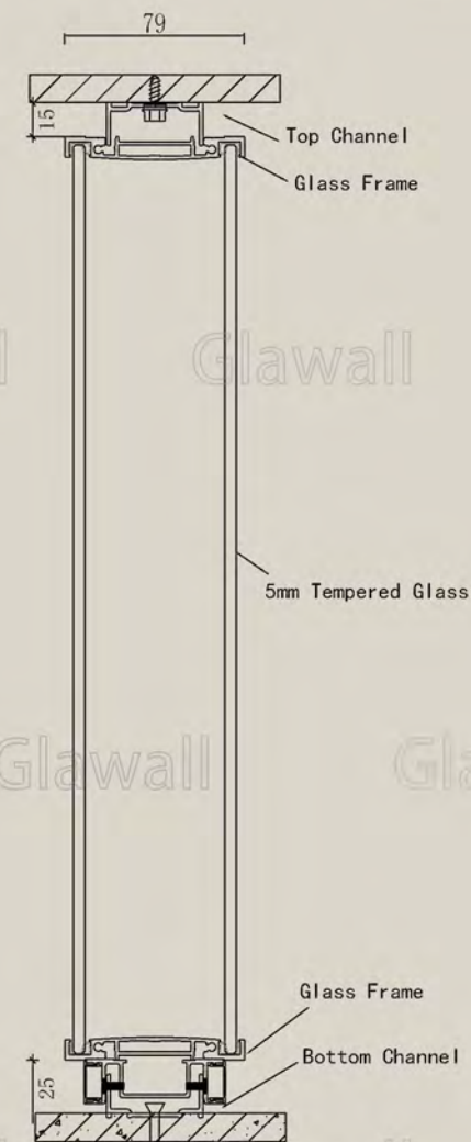
79 Series Double Glass | Panel THK: 79mm
