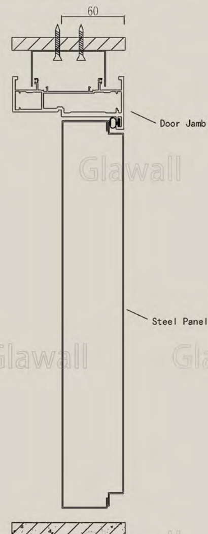
60 Series Steel Door | Panel THK: 60mm
